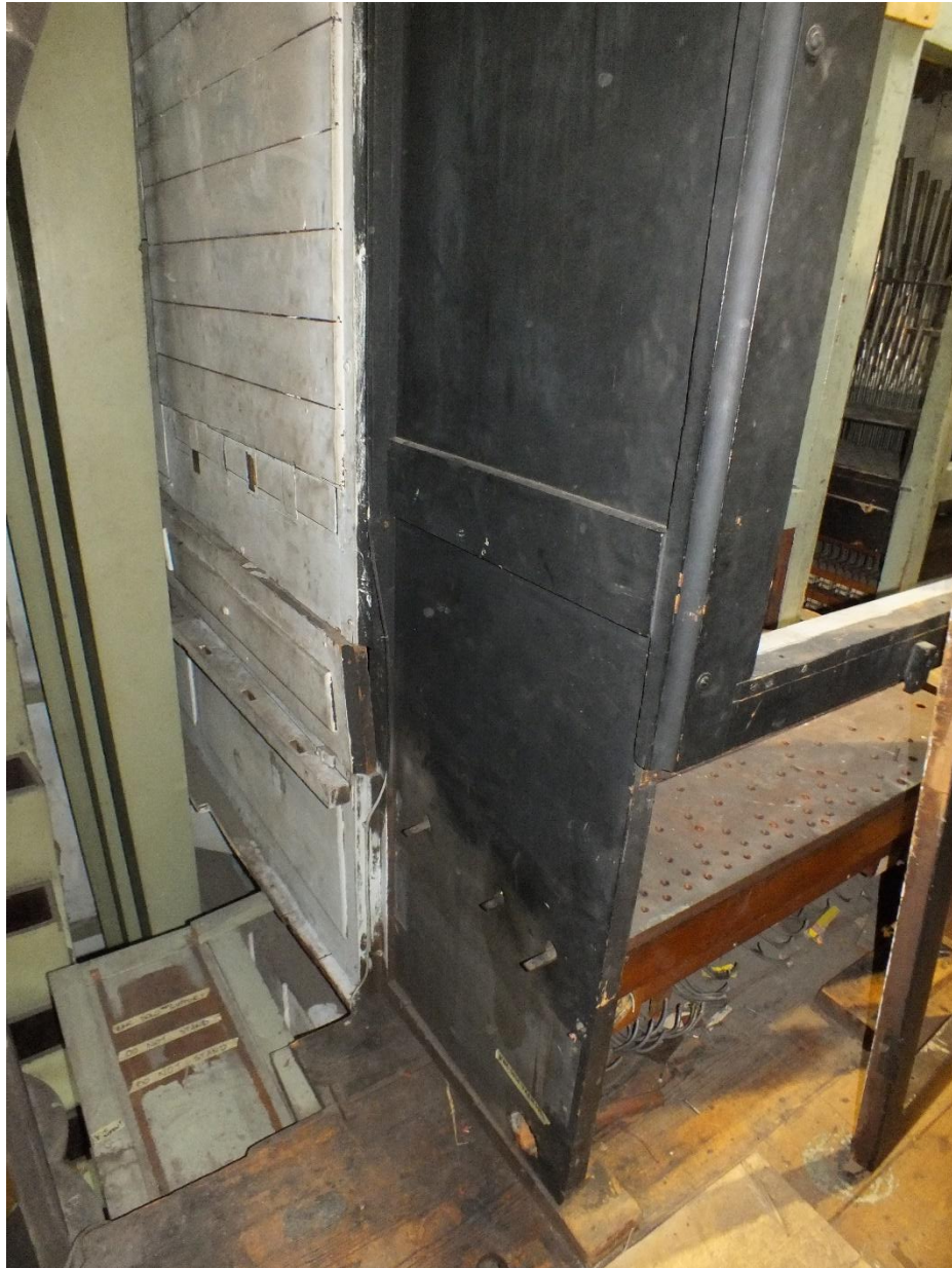
Forwards extension of Récit box for Enclosed Solo (shutters removed)
