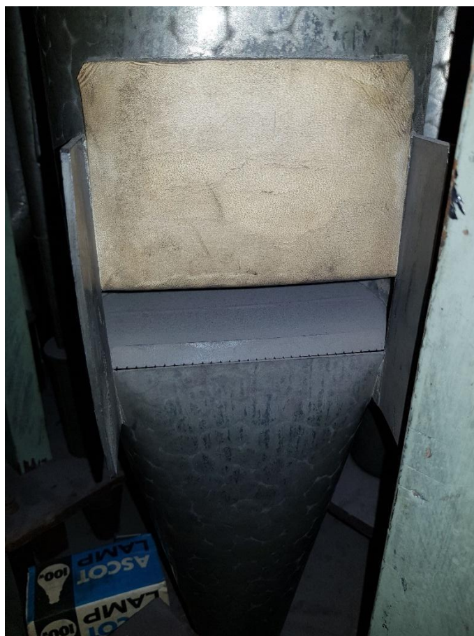
Leathered upper lip of 1913 Lewis & Co. Diapason Stentor 8'
