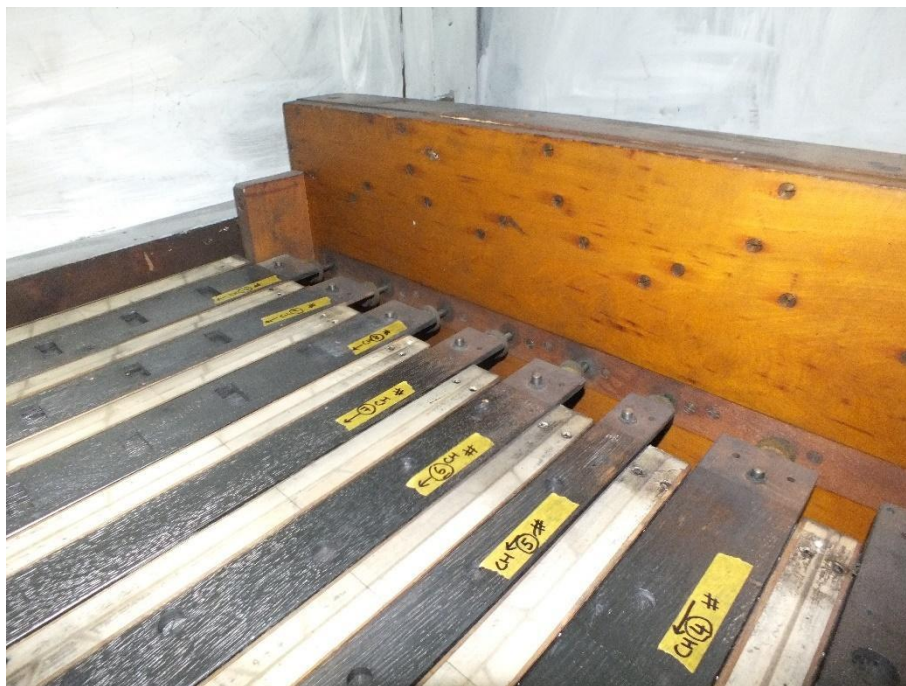
1913 Lewis & Co. pneumatic slider machine at rear of Positif C# soundboard
