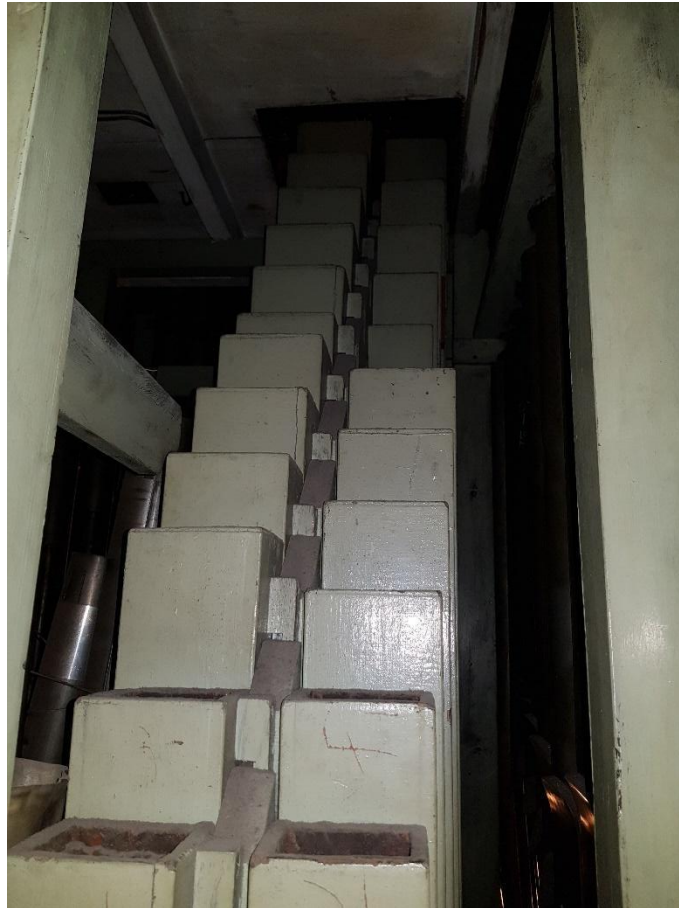
Grand Orgue C# off-note block for Bourdon 16', Bourdon 8' and Flûte Harmonique 8', every surface coated with 1970 green gloss paint
