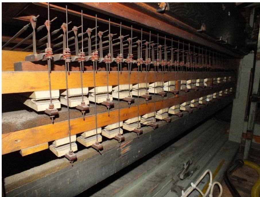
1913 Lewis & Co. pneumatic underaction beneath Récit C# soundboard Visible at top of image is the cross-trackering to the jeux de fonds pallets
