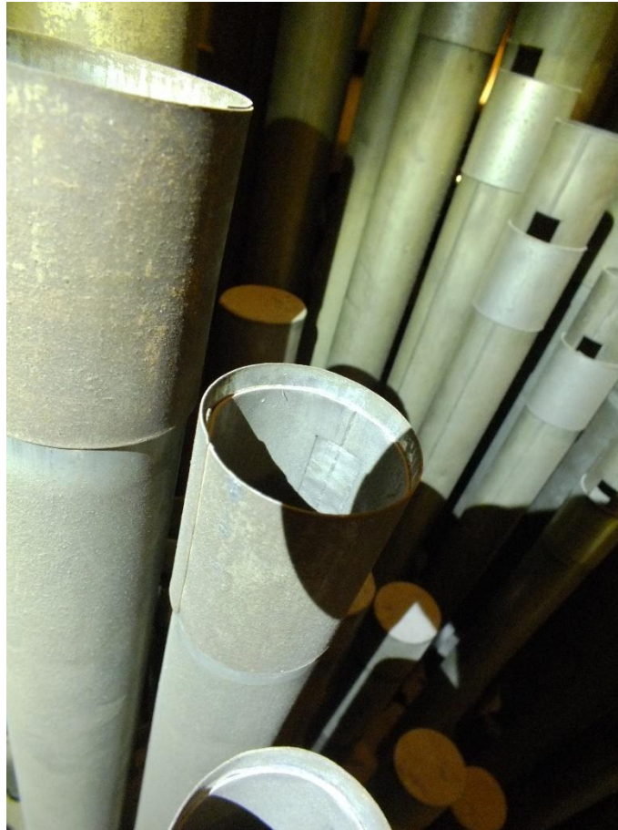
pipe has been cut, tuning slot soldered closed, tuning slide fitted, but note also the tide mark beneath the slide, suggesting that it is in its second position
