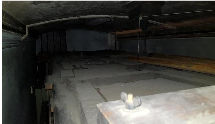
Upper of two enormous reservoirs squeezed into organist's retiring room in 1910
