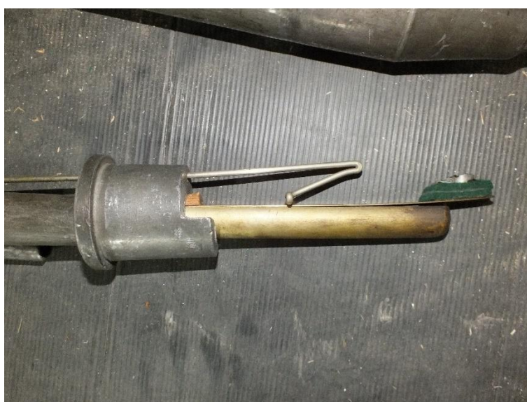
Non-original load applied to Pédale reed tongue
