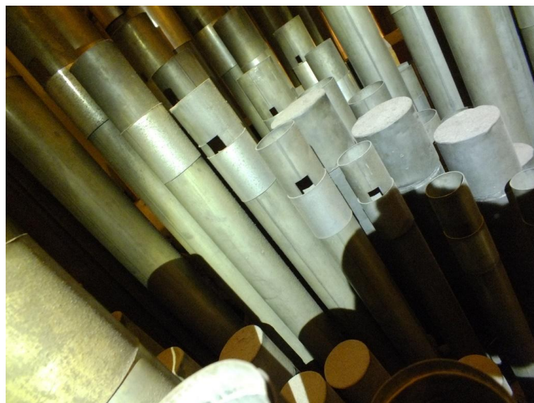
tuning slides added to shorter pipes
