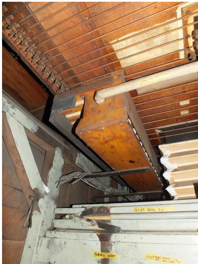
1913 Lewis & Co. pneumatic underaction for Pédale pallets in Grand Orgue soundboards
