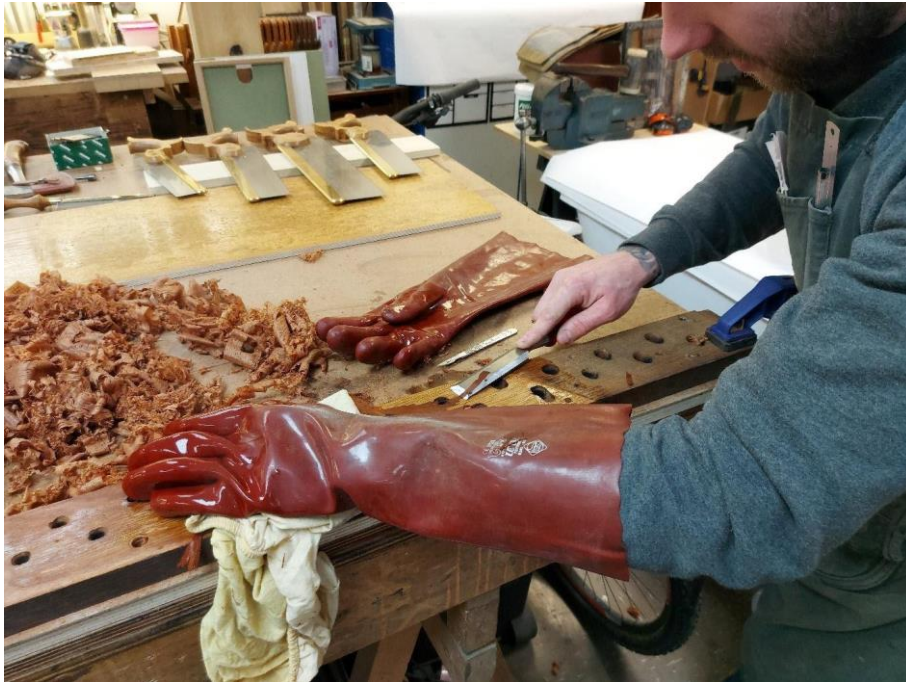
Using a hot damp rag and chisel to remove the remnant veneer after cutting and planing
