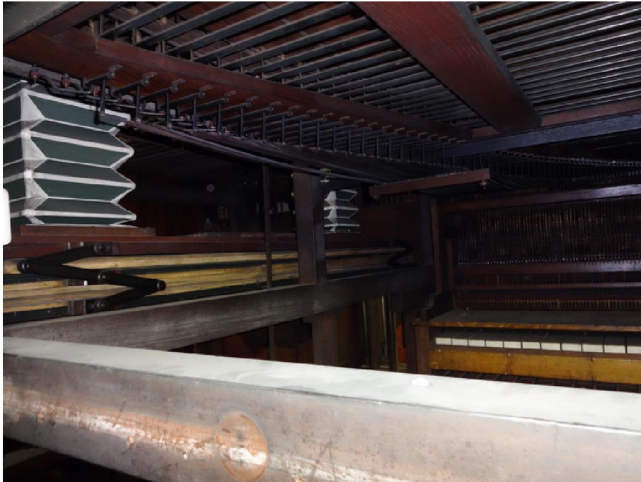
Horizontal rollers beneath soundboard at St-Antoine des Quinze-vingts, Paris
