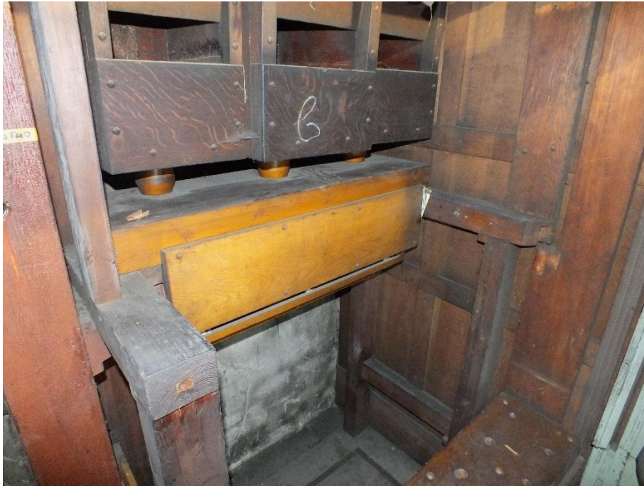
1913 Lewis & Co. chest for notes C1, D3 and E5 of the Soubasse 32' / Bourdon 16'
