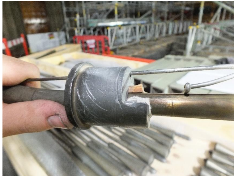
Shallot pulled out from original position in block and packed
