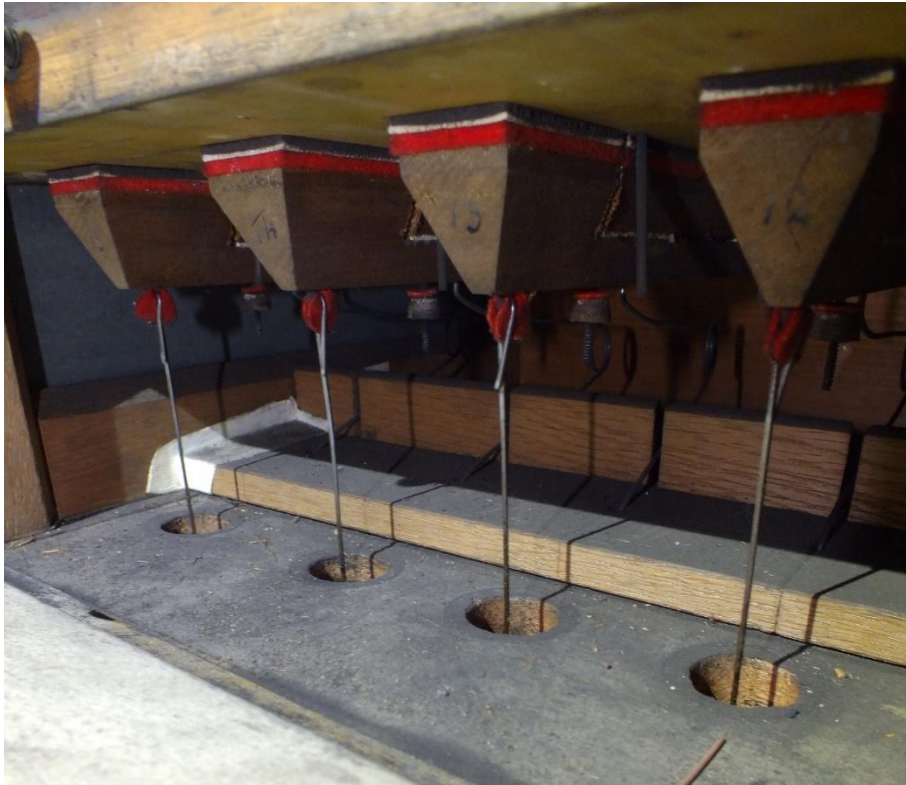
Pallets inside Récit soundboard showing L-shaped cuts to convert them to split form
