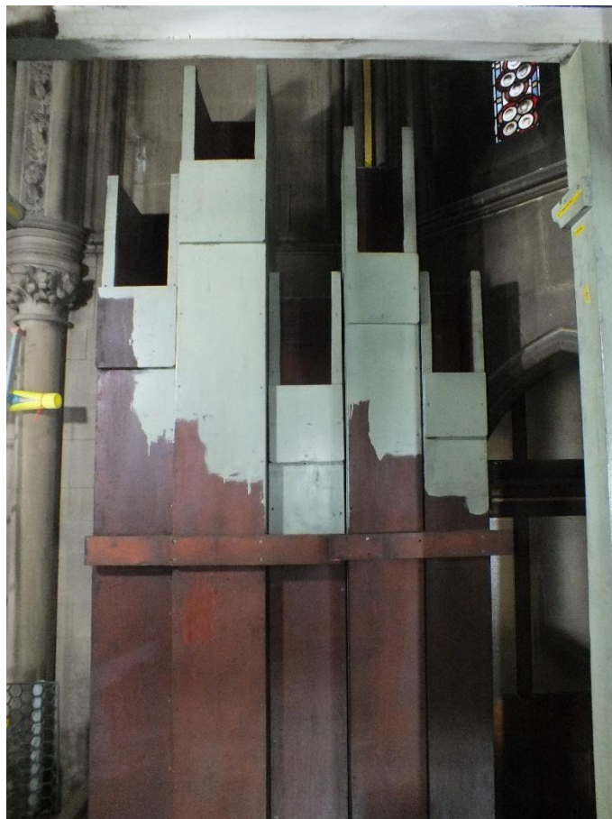
1893 Cavaillé-Coll Soubasse 32' / Bourdon 16' C# side pipes, re-made as Great Bass 16' / Octave 8' 1913 by Lewis & Co., part-painted gloss green 1970 by Jardine & Co.
