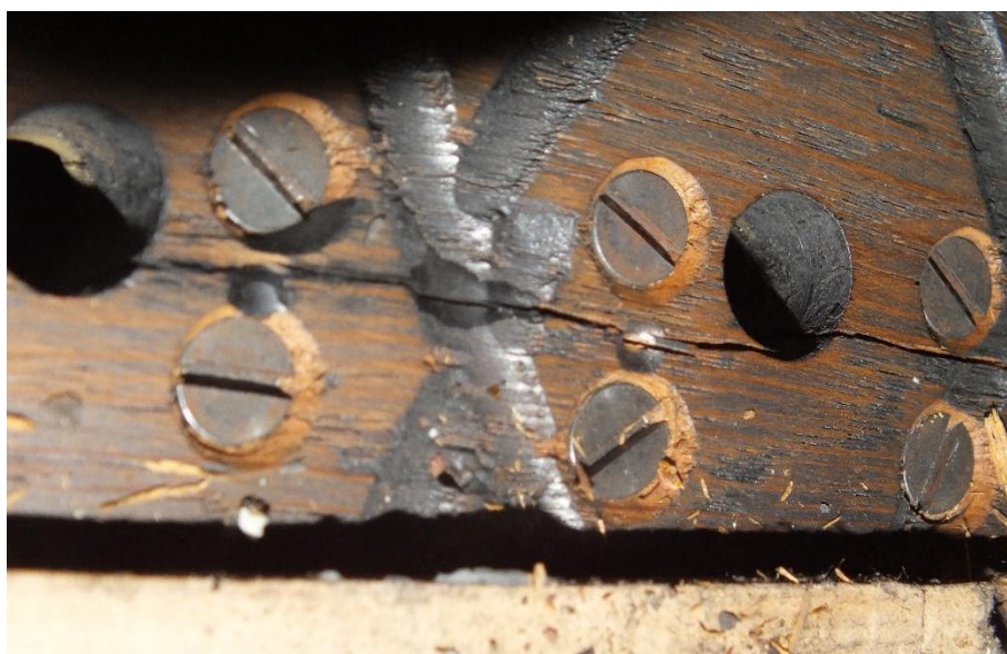
Previous repairs to split in Solo soundboard table
