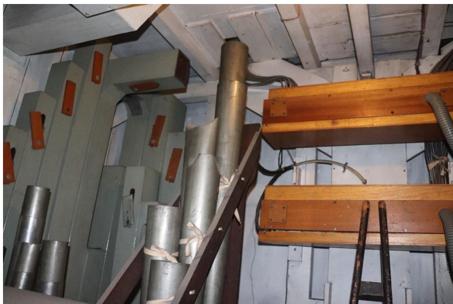
1970 Jardine & Co. change-over machines in Positif expression box, feeding the 1913 Lewis & Co. pneumatic underactions for the Récit on the floor above
